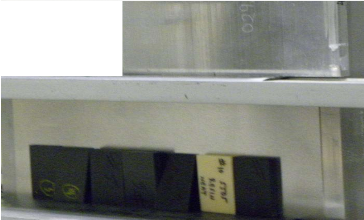
Figure 6. Optical image of small coupons with Borated Aluminum
