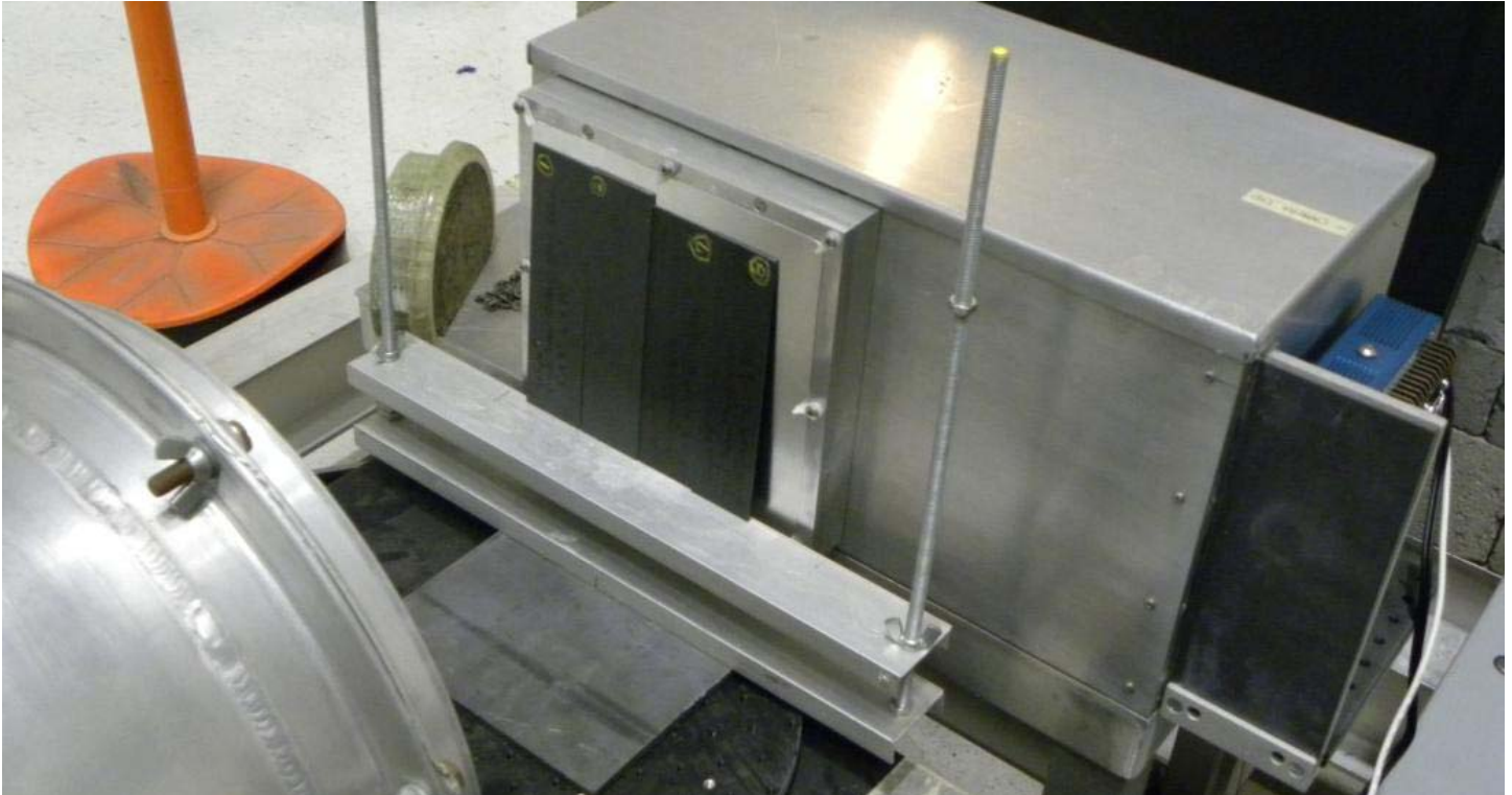
Figure 1. Neutron Radiography Imaging Station with samples 1, 2, 7, 8
