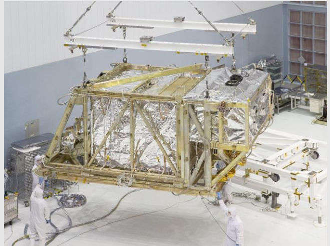
The ISIM connects via kinematic mount to the Primary Mirror Backplane with extreme precision. Composites produced with boron fiber, M55J, and K13C2U are used for both structural performance and zero CTE tuning.
