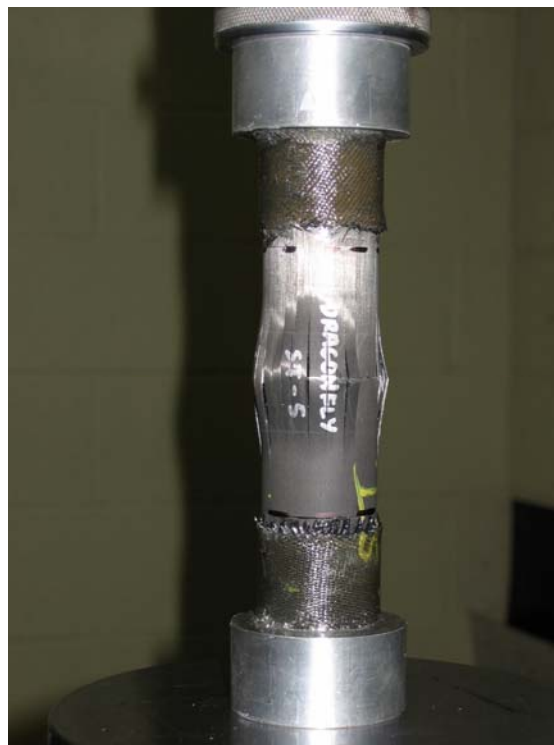
Figure 11. Hy-Bor Seat Tube After Compression Testing
