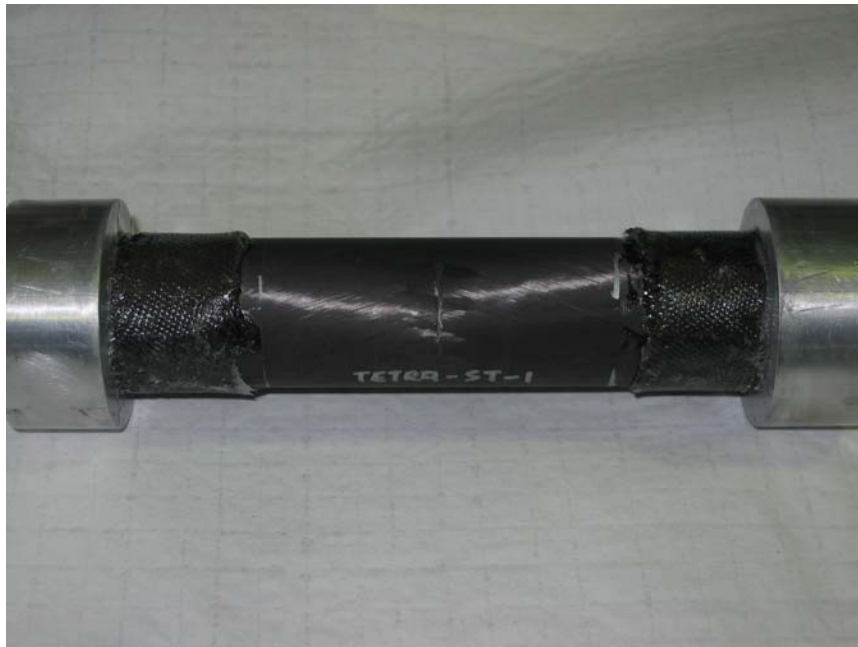
Figure 12. Graphite/Epoxy Seat Tube After Impact
