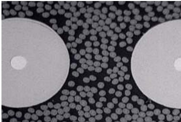
By combining carbon fiber with boron fiber, Hy-Bor<sup>®</sup> achieves the maximum compression strength of any continuous filament-based composite material. It can be tailored to meet specific materials properties and design objectives by customizing the graphite fiber and resin type and the boron fiber ratio.
