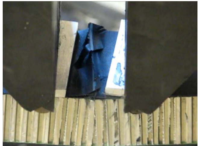
Figure 4. Failure phases of impacted Hy-Bor ® 208 specimens.
